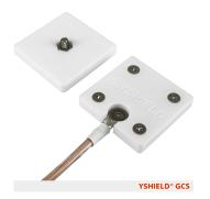
Grounding connection with two plates that get screwed together. For all electrically conductive fabrics, fleeces, meshes. The two connecting plates must be screwed together - the material that is supposed to be grounded needs therefore to be perforated.
